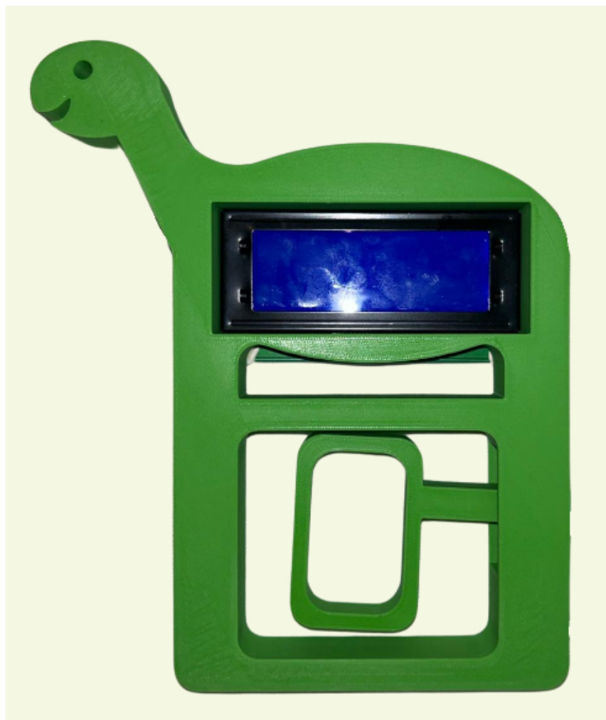
Figure 1. Preliminary prototype of the prototype device, constructed from 3D printing filament
